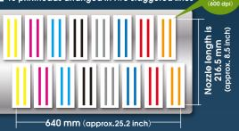
Tiger features 16 printheads (each line has 8 printheads) and allows a maximum high print speed of up to 385 m<sup>2</sup>/h\*. \* high speed (3 droplet size) mode 600 x 600 dpi, 1 pass, Bi; textile width ; 1.850 mm
