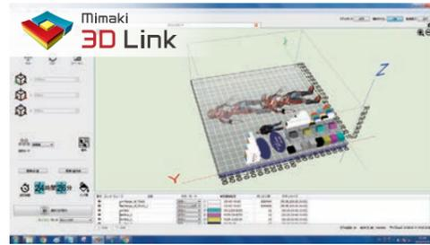
You can lay out your 3D data for printing and send the job data to the 3D printer.
