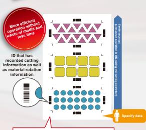
In the ID Cut function, even if there are a large number of types of cut data, any operator performs manual operation only once at first!
