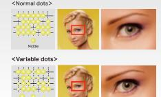
Dots are combined with the minimum size of 4pl to enable smooth color printing with less granular feeling
