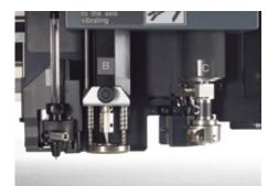
Thick materials up to 20 mm (0.78 ") can be cut with the reciprocating cutter. The R1 head is equipped with a material-holding unit, which prevents cut materials from lifting. The cutting head is suitable for cutting corrugated boards and foam materials.
