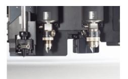
The tangential cutter steers the blades as it cuts. With two types of tangential cutters and fine cut pressure settings a wider range of materials can be cut successfully. Various cutting tools are provided for a range of materials. Any suitable blade available on the market, can be mounted.
