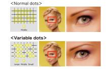
Dots are combined with the minimum size of 4pl to enable smooth color printing with less granular feeling.
