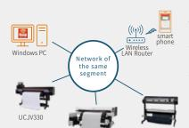
List ink type, heater temperature, and notification alerts on a smartphone or Windows-based PC.
