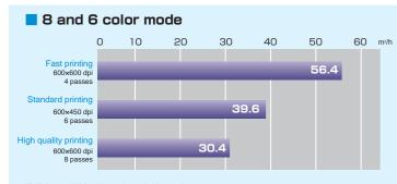
\*1 High speed, bidirectional printing in high precise drop mode \*2 When belt encoder revision function is used on Tx400-1800B, print speed decreases appr. 20%
