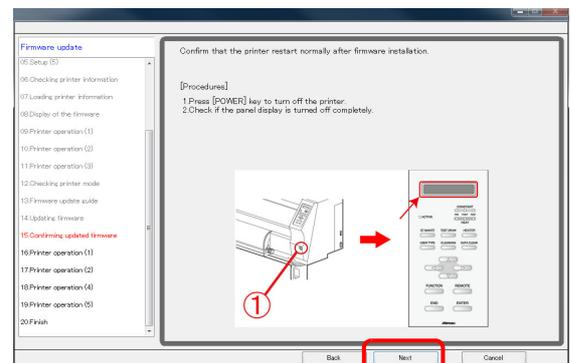
**29** Turn OFF the main power switch of the printer.
