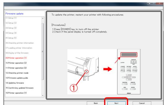
**17** Turn OFF the main power switch of the printer.
