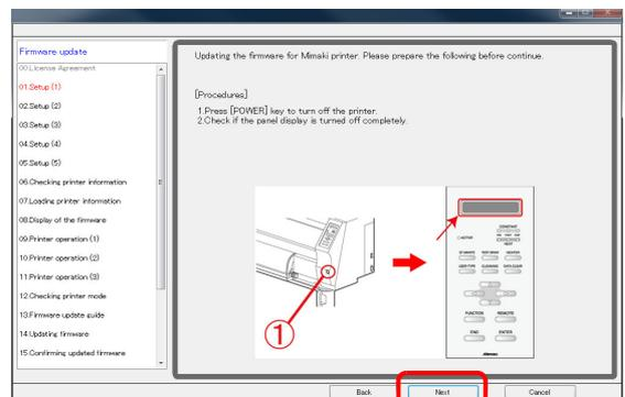
**6** Turn OFF the main power switch of the printer.
