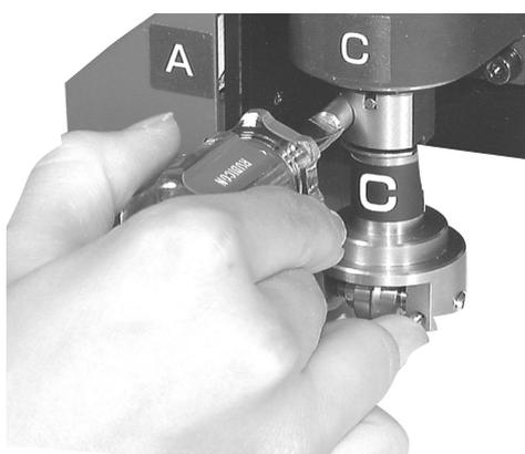
**Tighten the stopper screw with the screwdriver supplied with the device as an accessory.**
