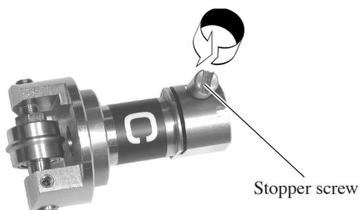
**Loosen the stopper screw in the crease roller.**
