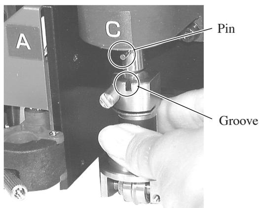
**Insert the pin of head C into the marking roller while fitting the pin in the groove on the roller.**
