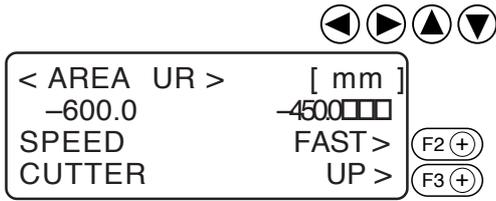
**Align the tip of the tool to the upper right point of the desired cutting area.**
