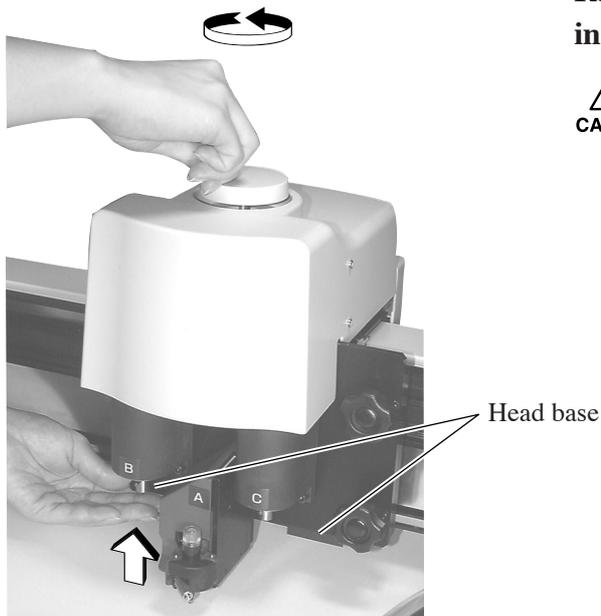
**Raise the head using the height adjusting knob.**
