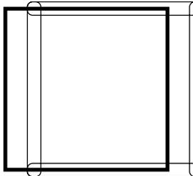
A square sample pattern is shown with a roller positioned to its left. The roller's edge is shifted towards the left side of the pattern, indicating a deviation to the left. |
