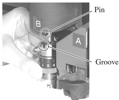
**Insert the pin of head B into the tangential cutter while fitting the pin in the groove on the cutter.**
