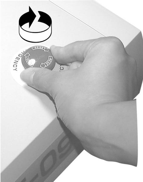
**Turn the EMERGENCY button clockwise for unlocking.**
