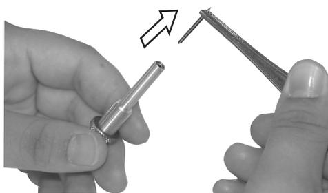
**Replace the blade tip with a new one using a pair of tweezers.**
