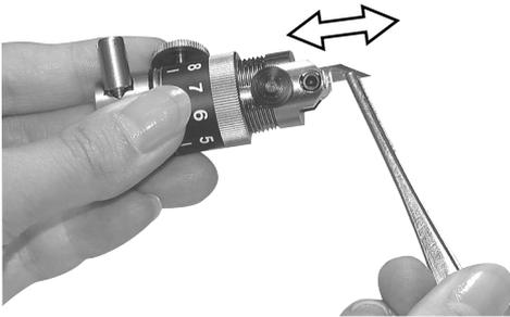
**Replace the blade tip with a new one.**
