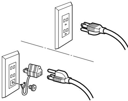
**Insert the other end of the power cable into the 3P receptacle.**
