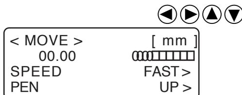
**Move the head to a position where test cut is to be performed.**
