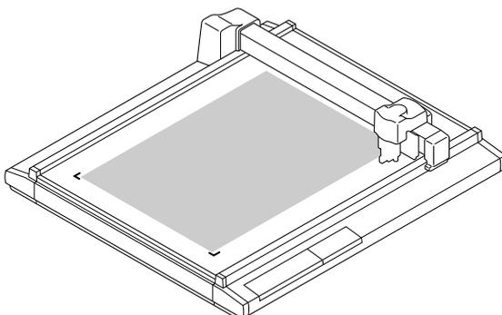
**Place a work on the cutting panel.**
