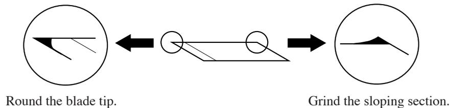
Gently rub the blade tip with the hand lapper while checking how far it is ground.
