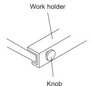
2. The right and left work holders may be turned upside down as needed according to the work size.
