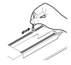
9. Check the flushing tray ink absorber. Replace if ink is found on the ink absorber.
