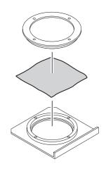
3. Install the filter holder on the filter unit.
