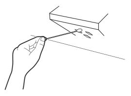
The ink cap prevents clogging of the head nozzle caused by dried nozzle.
