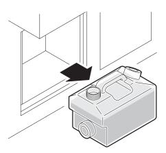
3. Put the empty waste ink tank back in the machine. The ink discharge way may become clogged by coagulated ink. It must be cleaned at regular intervals to avoid clogging.
