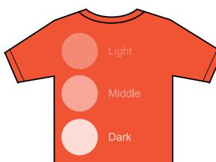
For ordinary printers, a dark portion of the image is printed darkly. However, as a result of printing with the discharge liquid and postprocessing, dark portions of the original image are printed light, and light portions are printed darkly. That is, contrasting density of original image appears inversely. Therefore, the image to be printed requires and black inversion before printing.
