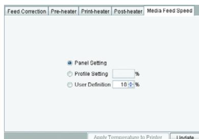
If the default Media Feed Speed does not feed correctly, set a value for Media Feed Speed.
