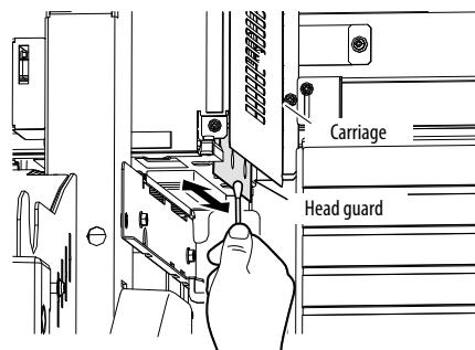
Clean the head guard at the right and left sides of the carriage using a cleaning swab or a soft cloth.
