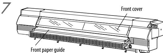
If the Printer is smeared with dust and paper dust, remove them using a vacuum cleaner. If the contamination is heavy, wipe it out with a soft cloth moistened with neutral detergent.
