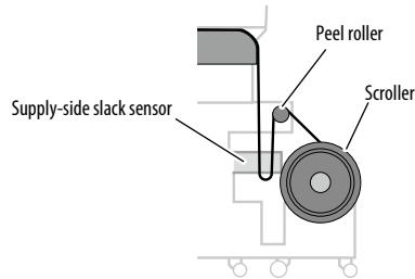
Slacken off to a level lower than the supply-side slack sensor. When the slack reaches the sensor detection area, the operation panel blips.
