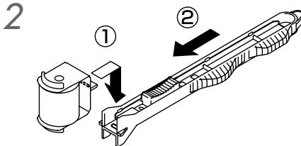
Attach the cleaning roller to the cleaning stick.
