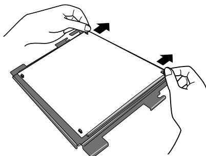
Remove all wrinkles on the head cleaning sheet by lightly pulling both sides of the sheet top edge in the direction of the arrows. This will prevent the sheet from rising near the bottom edge attachment locations.
