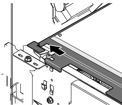
Install the sheet cleaning part you prepared in advance to the wiping unit.
