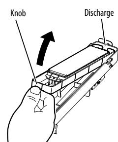
Press the knob at the near side of the case containing the spittoon absorber liquid to open the lid, raise the front side of the spittoon absorber liquid case to discharge the spittoon absorber liquid to the backside.
