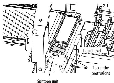
Confirm that the spittoon absorber liquid's top surface is as high as the top of the protrusions.
