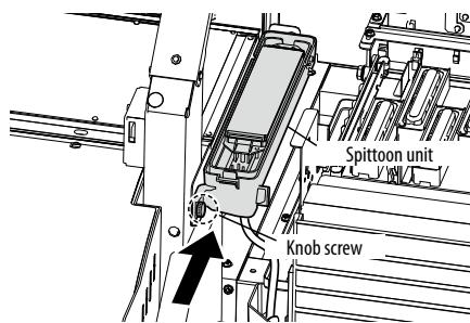
Install the new spittoon unit with the knob screw.
