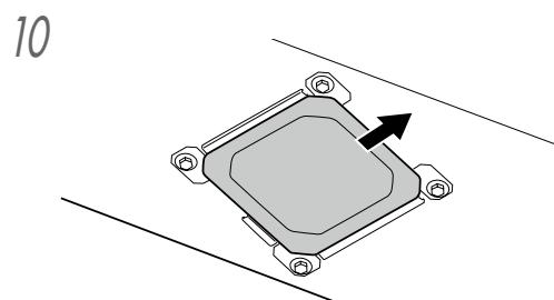
Remove the old exhaust fan filters.
