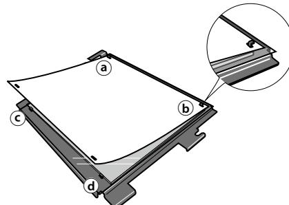
Place the head cleaning sheet on top of the support sheet. Hook two holes to the attachment locations (a) and (b) and then the two others holes to the attachment locations (c) and (d).
