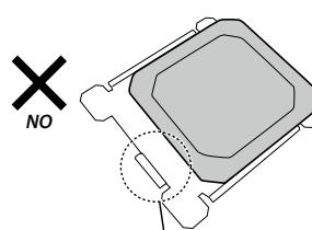
The filter does not touch the shorter filter guide.
