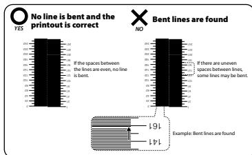
Check that there are no missing or bent lines.
