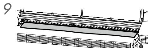
By installing an unnecessary media or cloth on the platen, prevent the Printer from being smeared with the dust accumulated on the exhaust fan filters.
