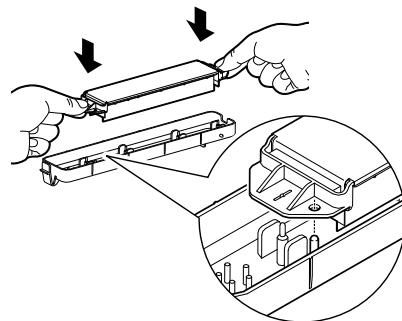
Set a new spittoon case's locating hole to the protrusion, and fix it horizontally by pressing slightly.
