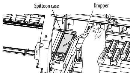
Moisten the spittoon case with the spittoon absorber liquid using a dropper.
