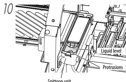
Pour the spittoon absorber liquid into the spittoon case until the liquid level is as high as the indication protrusions.
