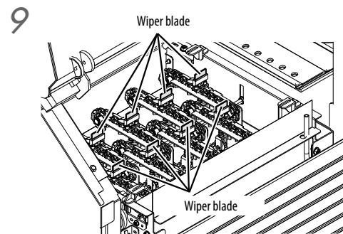
Visually check the wiper blade for contamination and scratches.
