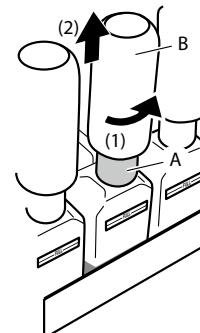
Turn slowly the B part in the counter-clockwise direction while holding the A part with your hand to prevent it from turning.
