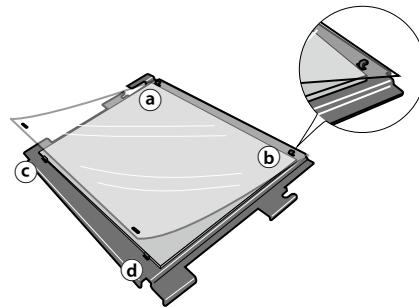
Hook two holes of the support sheet to the cleaning sheet mount attachment locations (a) and (b). Keep the sheet stretched and hook the two remaining holes to the attachment locations (c) and (d).
