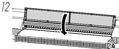
12 Remove the media or cloth installed at the step 3, and close the front cover.
