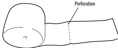
From a new filter roll, along perforation tear off the amount required for the replacement.
