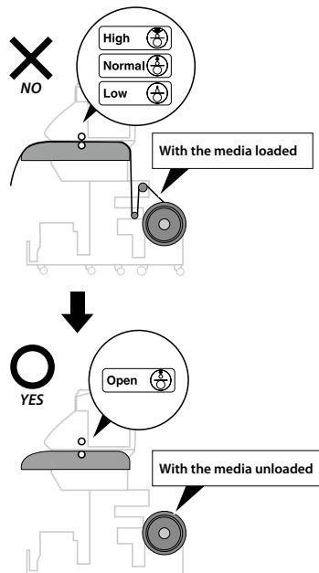
If you keep the media loaded on the Printer for a long time, the media may be wrinkled on the platen or the media gripping trace may be left. To keep the media in good condition, the operation below is recommended. Especially after printing on Vinyl, be sure to unload it from the Printer.
