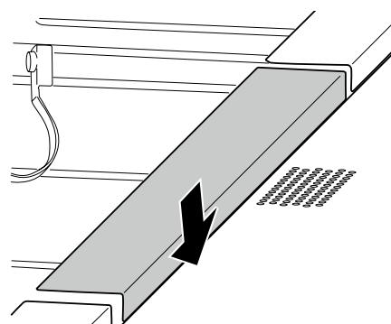
Remove the old suction fan filters from the hook-and-loop fastener.
