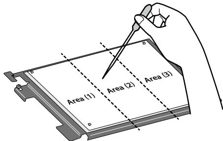
Apply 4 cc of wiper cleaning liquid on the head cleaning sheet surface using a dropper. Apply 1 cc four times as follows.
