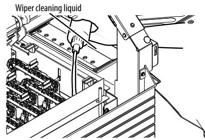
When the cleaning liquid level is lower than the "X" mark's top edge, replenish the wiper cleaning liquid.
