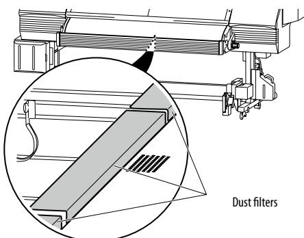
When replacing the dust filters from the operation panel menu, start the procedure from step 1. When replacing while executing [**#START MAINTENANCE**], start the procedure in step 6.
