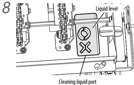
Check the wiper cleaning liquid level.
