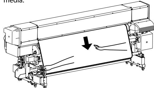
**6** Remove the scroller of the printer.
