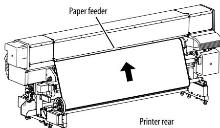
If it is hard to insert the media end into the paper feeder due to a curl of the media, interpose an interleaf and insert the media end under the interleaf as shown in the figure below.
