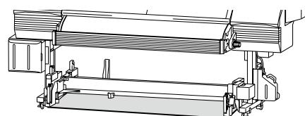
By spreading an unnecessary media or cloth on the floor, prevent the floor from being smeared with the ink clot dropped from the old suction fan filters.
