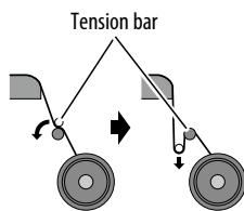
Adjust the tension bar length and decide whether to attach a flange or not, depending on the type and width of the media.
