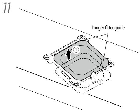
Install the new exhaust fan filters.
