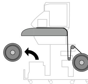
When the media is installed on the take-up reel unit, remove the media.
