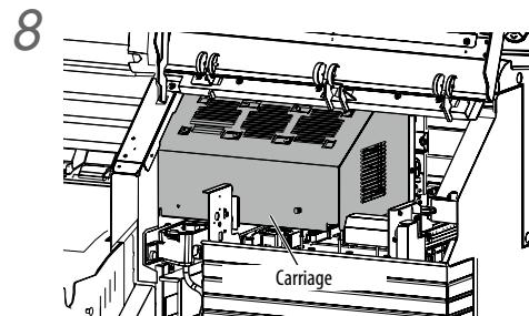
8 Vacuum the dust off the carriage's fresh air inlet. Monthly cleaning is recommended.
