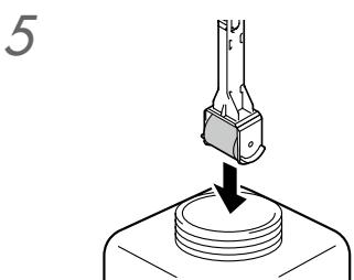
Soak the cleaning roller in the cap cleaning liquid.
