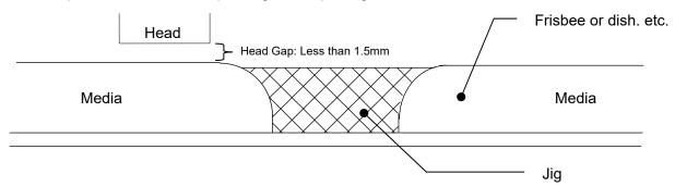
2. Please cover the blank space of the table to prevent the reflection of the UV light when printing on thick materials. (Make sure it does not interfere with the head and Y bar movement.)
