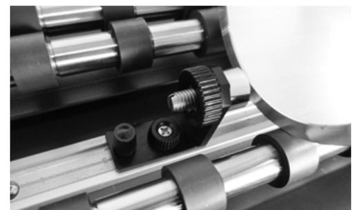
**10** Tighten the screw of the left work holder.
