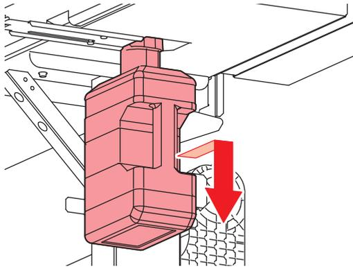
**6** Attach the cap to the removed waste ink tank, and use tape to prevent leakage of waste ink.
