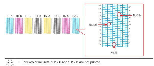
Select the "head number and nozzle row" for nozzle recovery, then press the [ENTER] key.
