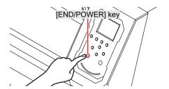
• Do not turn off the main power supply. Turning off the main power supply will disable the automatic maintenance function (including nozzle clogging prevention function and ink discharge channel cleaning function). This increases the risk of ejection failures (such as nozzle clogging or deflection).
