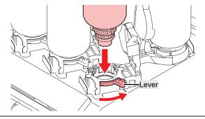
• You may apply the maintenance liquid onto the O-ring of the ink bottle caps so that the ink bottle can be inserted easily. Use the appropriate maintenance liquid to suit the ink being used.
