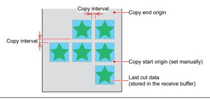
• The machine cuts the specified number of sheets of the divided cut data without separating the data.
