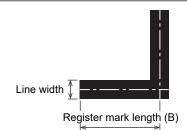
The recommended register mark length and line width are as shown below. The machine may fail to detect register marks that lie outside the recommended range.
