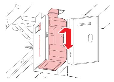
5 Attach the cap to the removed waste ink tank, and use tape to prevent leakage of waste ink.
