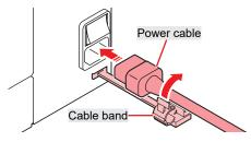
**5** Plug the power plug into the power outlet.
