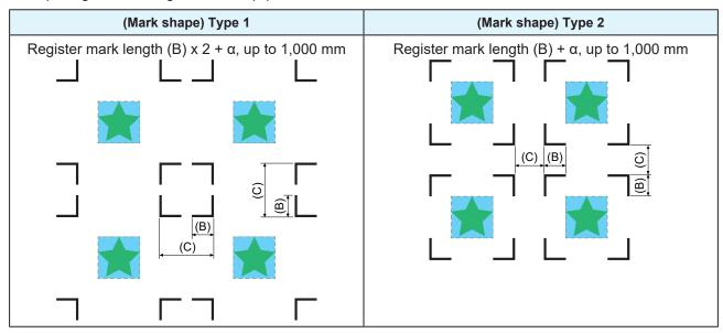
The spacing between register marks (C) is as shown below.
