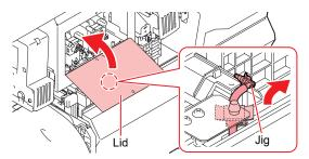
• Connect the jig by pushing the tip into the port and rotating 30° clockwise.
