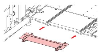
7 Secure the media holder stopper with the screw.
