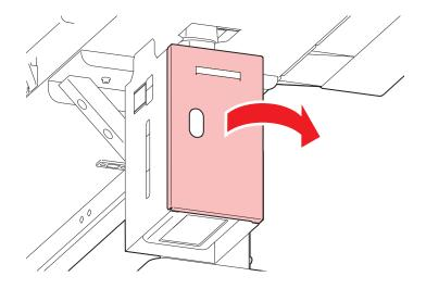
**4** Hold the handle on the waste ink tank and slide out.
