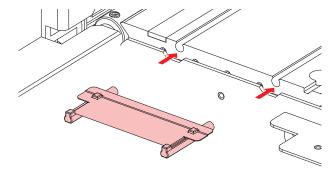
5 Secure the media holder stopper with the screw.
