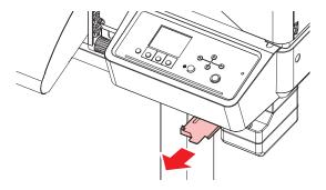
5 Hold the handle on the waste ink tank and slide out.
