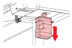
Attach the cap to the removed waste ink tank, and use tape to prevent leakage of waste ink.
