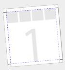
(2) After special color printing is finished, the skew angle is applied when ripping the regular color layer.
