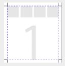
• Media is pulled back, the marks are detected, and the skew is calculated.
