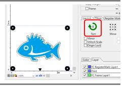
In the [Layer] tab, uncheck all layers except for those containing the coating data (cutting data) and register marks.
