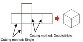
• When setting the double or triple above, [Z Remainder] and [Width to Fold] must be set so that the extension line of blade tip and the cut line in the data are aligned. Note that if these settings are different, the box shape will become corrupted.
