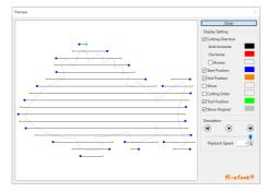
• Clicking the [Trace] button moves the head without printing the top coat, enabling the coating position to be checked without wasting media.
