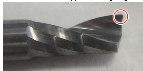
End mill with chipped cutting edge
