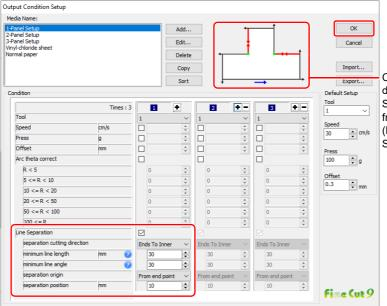
Check the Separation cutting direction and the Separation position changing from the Separation origin. (Displays only when [Line Separation] is selected.)
