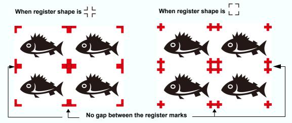
• On the CFL-605RT, set the same values as the settings above. Setting items of each machine: [SIZE] [STYLE] See the operation manual of each machine for details.
