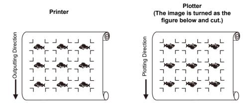
(1) After the step 2, click the Turn button to 180 degrees in the [Layout] tab.
