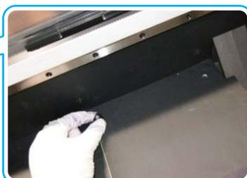
Loosen up the screws (for four positions) and remove the cover.
