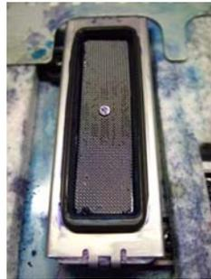
**Important!** • After cleaning, make sure that the cap rubber and mesh in the cap are not removed.
