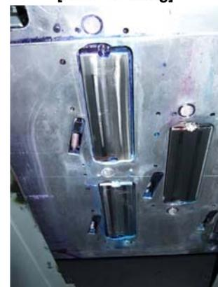
**Important!** • When you leave during maintenance (or cleaning), please make sure to complete the cleaning by pressing **ENTER** key. Without completing the cleaning, the nozzle part is left uncovered and then outside light makes the ink cure, which causes nozzle clogging or the like.
