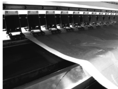
The media on the ink receiver is slack. Adjust it.
