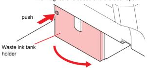
(2) By holding the waste ink tank, pull the tank to remove.
