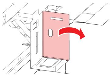
▲ Hold the handle on the waste ink tank and slide out.
