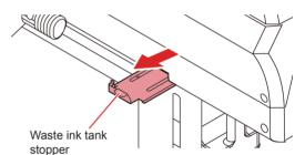
Pull it frontward to remove by holding the waste ink tank handle.
